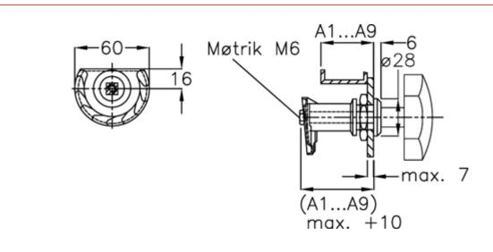
Door + frame thickness = 47-55 Measure type = A7
